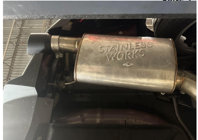
Detail 12a: Left muffler assembly installed
