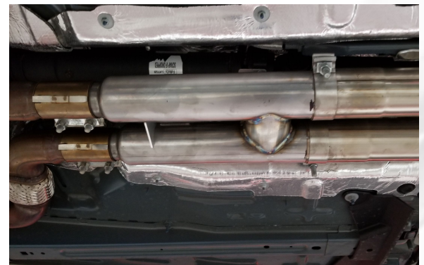
Detail 9: H-pipe and mid pipes installed (factory connect shown)
