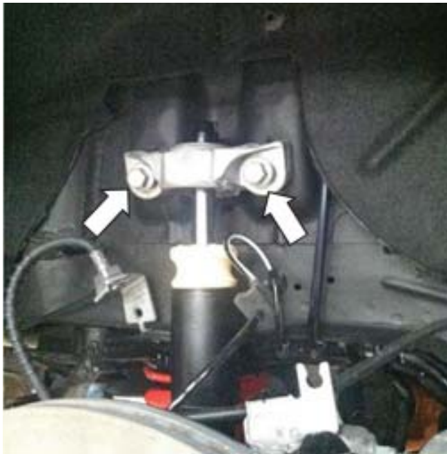
12. Go back and tighten the two (2) lower shock bolts to 48 Nm using a 15 mm socket. Remove the jack.
