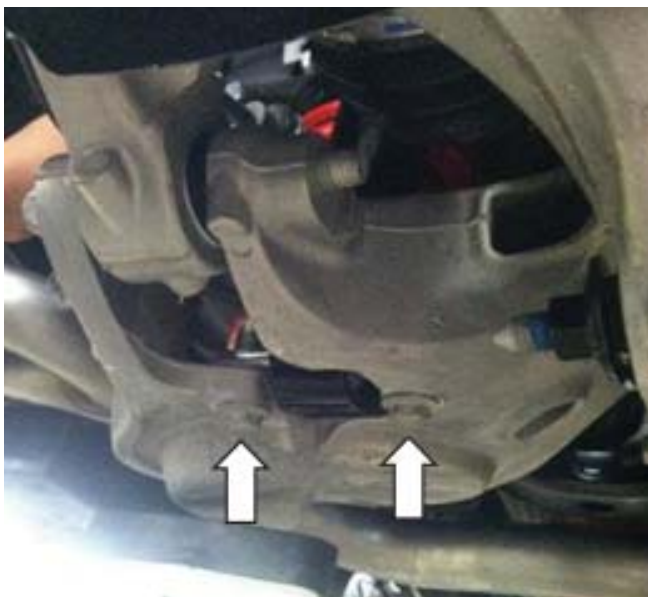
13. Use a 13 mm socket to refasten the brake line bracket back onto the frame. Torque to 10 Nm.
