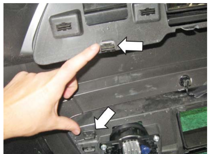
Close up of the outer two (2) J-clips installed (right/passenger side shown). Notice how they are installed in the opposite orientation from the rest (upside down)
