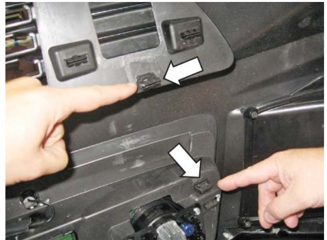
Be sure to engage the tabs on the top side of the splitter to the fascia
