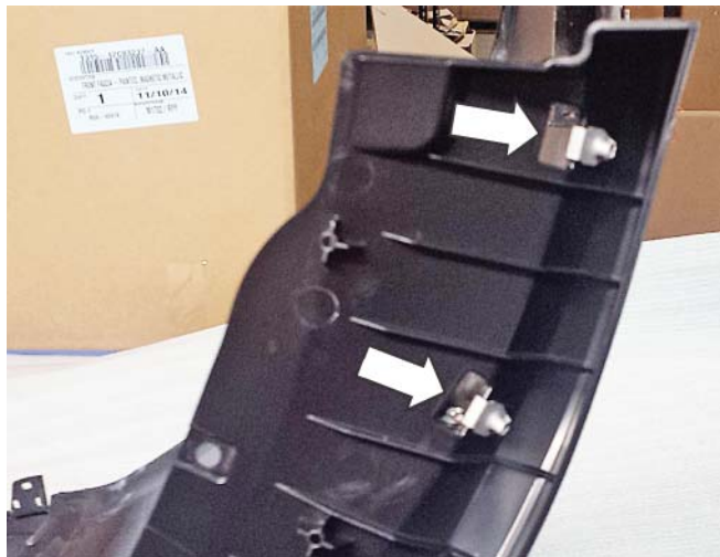
Close up of the outer two (2) J-clips installed (right/passenger side shown). Notice how they are installed in the opposite orientation from the rest (upside down)
