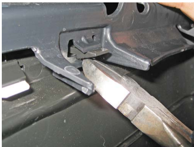
Close up of the retaining clip engagement
