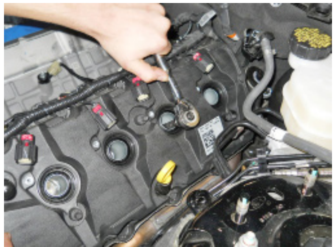
15. Unpack the eight (8) provided spark plugs (M-12405-M50), YOU MUST RE-GAP PLUGS TO 0.9 mm (.035") and verify that the plugs are not damaged.
