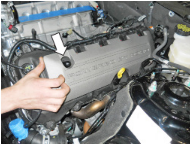
11. Disconnect the electrical connectors for each of the ignition coils.
