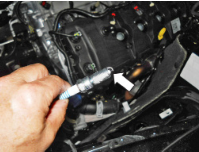
16. Install the spark plugs and torque to 14 Nm.
