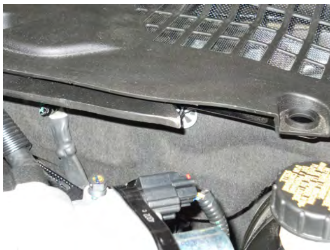
Exposed point on modified K-brace, shown installed
