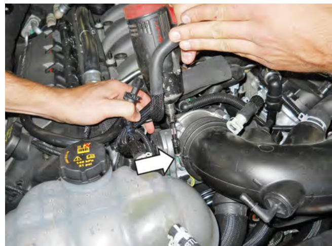
Clamp at throttle body
