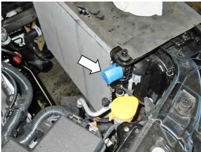
60. Tape off the radiator hose port and inlet port.
