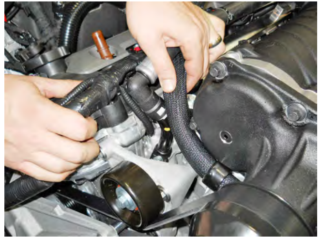
Outlet hose moved to show hose plug underneath
