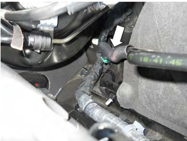
Disconnect green quick connect fitting
