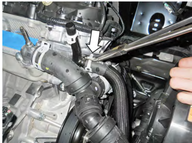
Degas hose from bottom of bottle
