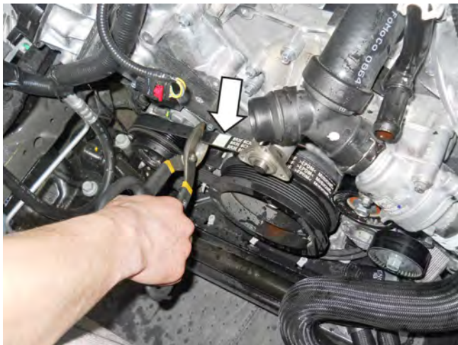
52. Cut and remove the A/C compressor belt. Discard belt.
