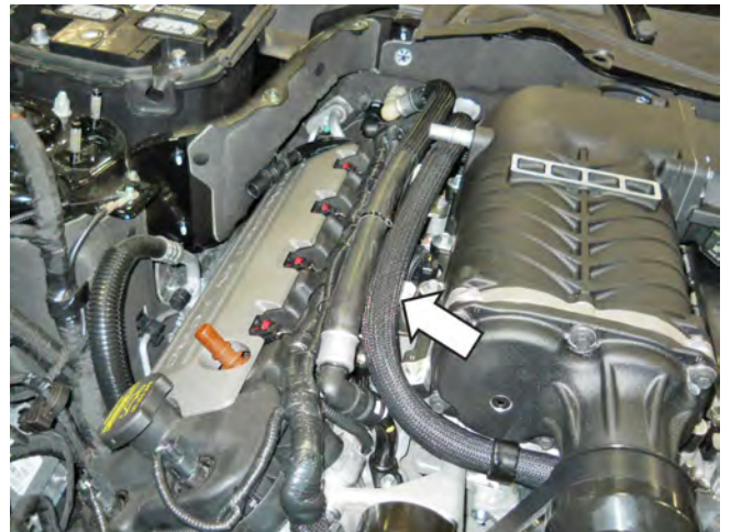
43. Secure the heater inlet hose to the new heater outlet hose assembly with zip ties.
