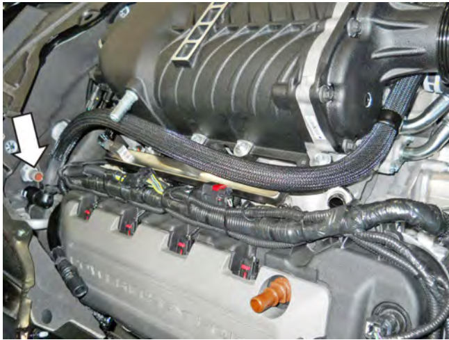
40. Install the heater hose connector to the bottom port (heater outlet) at the RH firewall.
