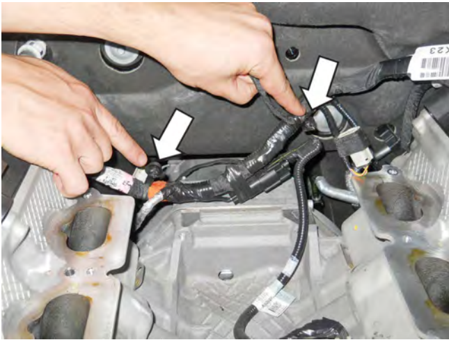
Pin retainers on harness
