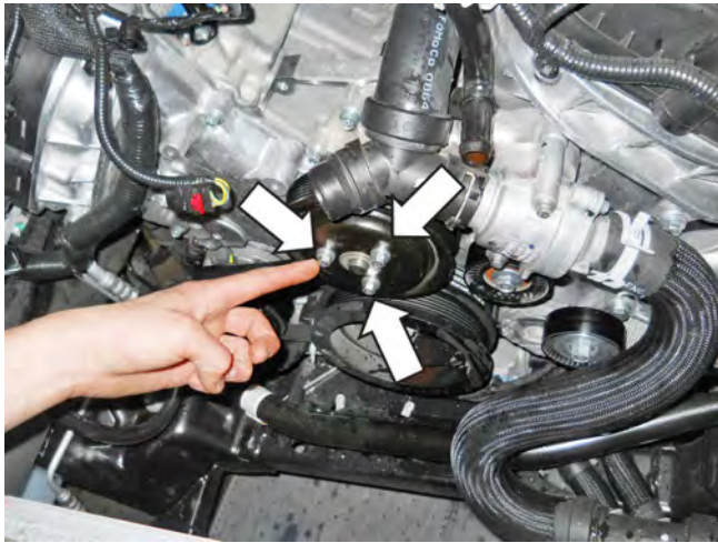
52. Cut and remove the A/C compressor belt. Discard belt.
