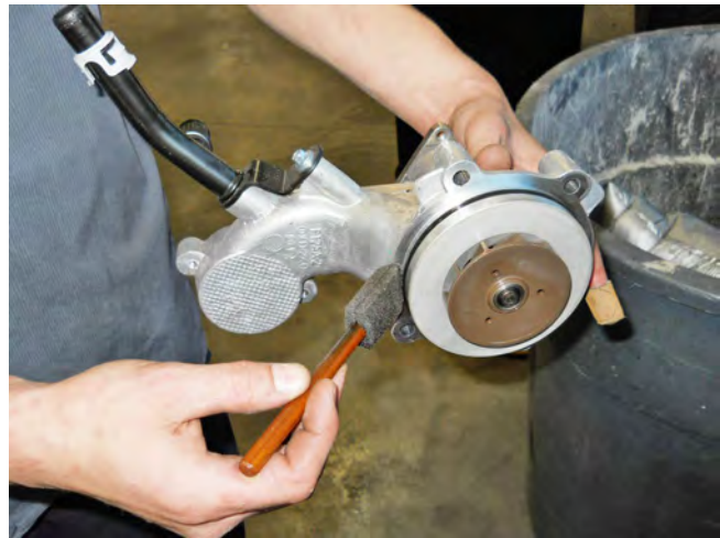
3. Install the water pump on the front cover and install the three (3) bolts only. Leave out the bolt at the 10 o'clock position. Torque the bolts to 25 Nm.
