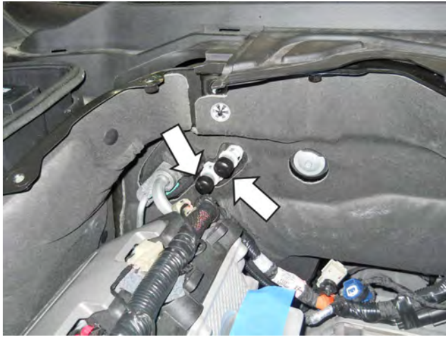
60. Tape off the radiator hose port and inlet port.
