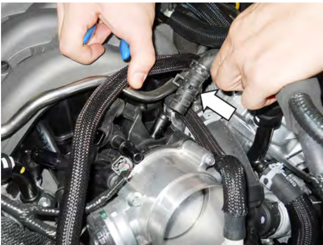
30. Move the LH heater hose aside from the support bracket on top of the LH cylinder head.
