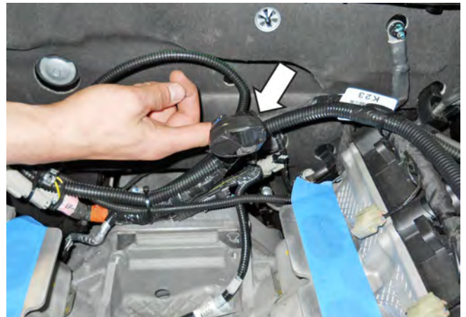
CMCV connectors taped up
