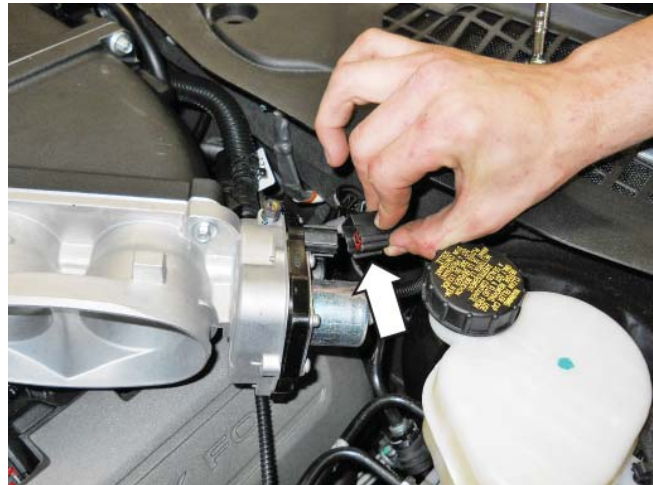
20. Install the ETC and TPS electrical connectors to the throttle body.
