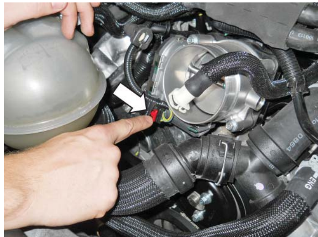
31. Unlock the green connector and disconnect the evaporative emission canister purge valve (EECPV) tube and electrical connector (green). Remove the EECPV tube retainer from the front left hand cam cover. Disconnect the remainder of the tube at the fitting located behind the inner passenger side fender. A fuel line removal tool will be necessary to release the connector. Remove from vehicle and set it aside. Both connectors will be transferred to the new line in Hardware Kit E Wiring. (Pictures show left hand drive model. Line routing may vary.)
