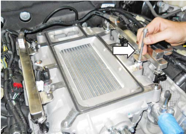
8. Connect the eight (8) fuel injector electrical connectors.
