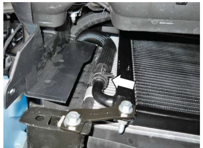
Pump hose to LTR connection
