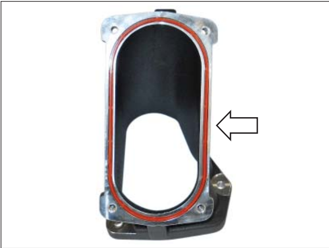
17. Mount the throttle body spacer (1315-9P697) using four (4) M6 x 32.5 fasteners (R18020009). These parts can be found in Hardware Kit B (1315-TVSHKB). Torque the fasteners to 10 Nm.
