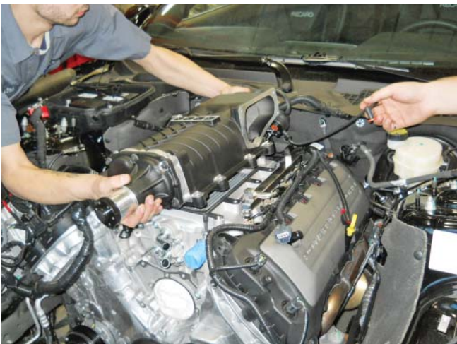
9. Carefully place the supercharger assembly (1315-6F066) on top of the intake manifold. Ensure that the supercharger is fully seated on the intake mounting dowels. Remove protective shipping covers.
