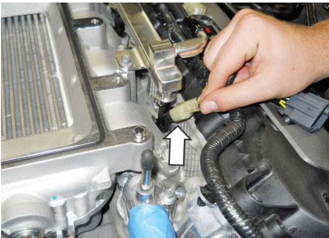
9. Carefully place the supercharger assembly (1315-6F066) on top of the intake manifold. Ensure that the supercharger is fully seated on the intake mounting dowels. Remove protective shipping covers.
