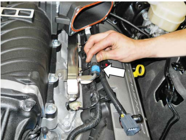
18. Connect the fuel supply line to the fuel rail and lock it into position.
