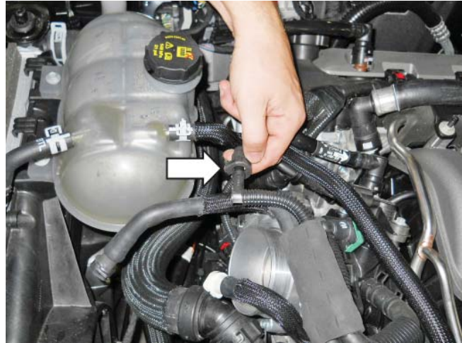
30. Disconnect the throttle body electrical connector. Pull the red locking tab back; press the black release tab to disengage the lock.
