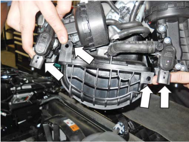
Harness pushpin retainer points on rear of intake
