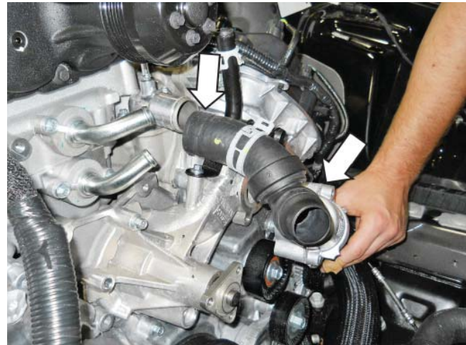
5. Install the two (2) thermostat housing mounting bolts and torque to 10 Nm.
