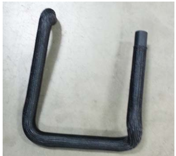
Intercooler pump outlet hose (1315-6K236)
