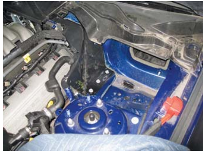
8. Release the eight (8) pushpin retainers by pulling the center pin and remove the radiator trim cover.
