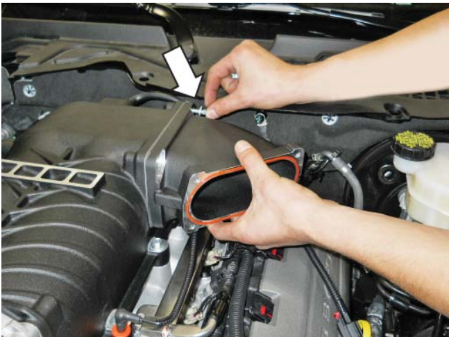
18. Connect the fuel supply line to the fuel rail and lock it into position.
