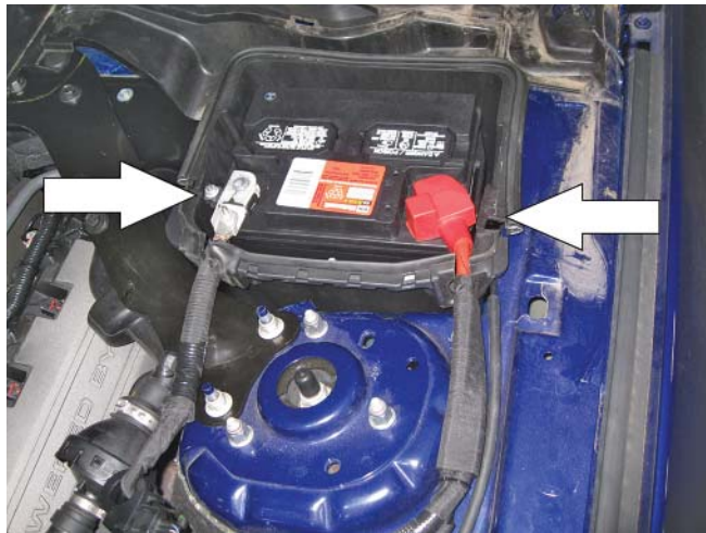
5. Remove the tie down battery clamp.
