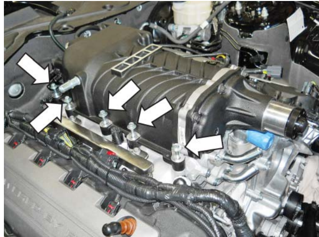
10. Install the ten (10) M8 x 1.25 x 53 fasteners (N808130) provided found in Hardware Kit B (1315-TVSHKB) into the mounting holes. Torque fasteners to 25 Nm in the sequence shown (10 mm socket).
