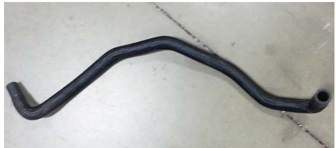
Intercooler pump inlet hose (1315-8D029)
