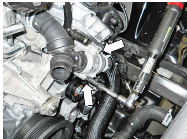
5. Install the two (2) thermostat housing mounting bolts and torque to 10 Nm.
