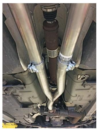
Tighten front clamps to 48 Nm. Tighten the rear clamps to 55 Nm.
