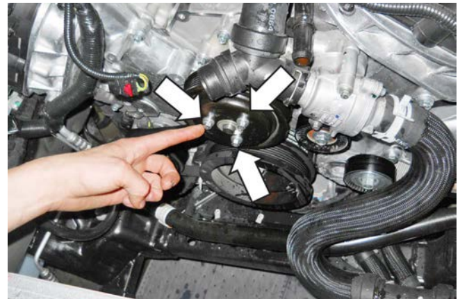
43. Cut and remove the A/C compressor belt. Discard the belt.
