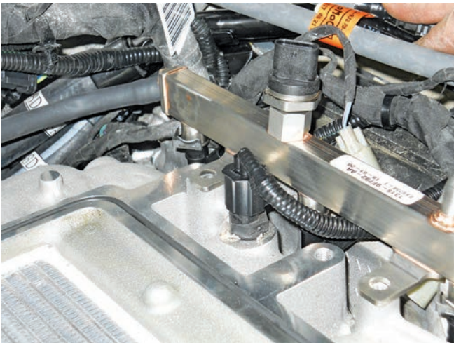
12. Lubricate the lower fuel injector O-rings with petroleum jelly or engine oil. Install the fuel rail and injectors into the intake manifold. Be sure each injector is properly seated into the intake manifold. Leave passenger side loosely installed. Install the one (1) previously removed fuel rail mounting bolts into the fuel rail mounting locations (5) in the figure below.
