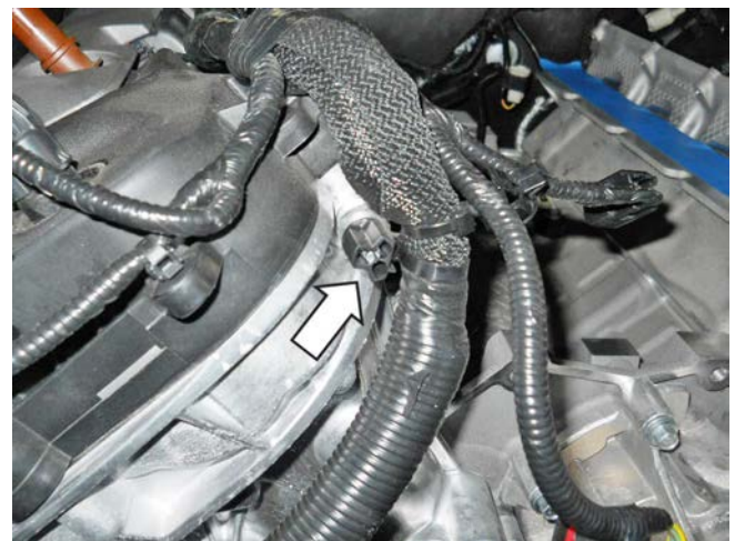
45. Cap or tape off the PCV port, heater feed tube.
