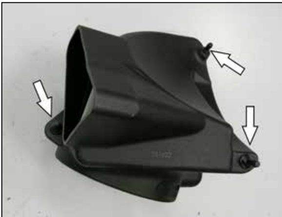
13. Install the provided mounting studs onto the K&N air filter housing using the provided hardware.
