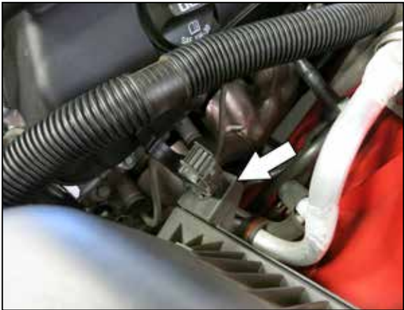
5. Disconnect the sound tube from the factory air filter housing.
