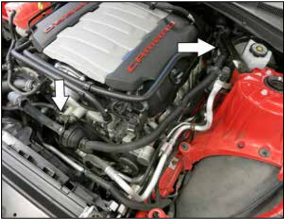
6. Remove the complete factory intake system from the vehicle.
