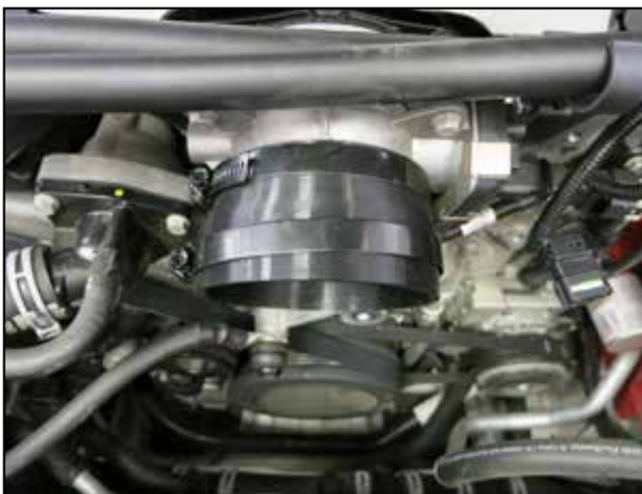
15. Install the provided coupler onto the throttle body with the provided hose clamps. Tighten clamps using 5/16" socket or nut driver. Note: Do not over tighten clamps.
