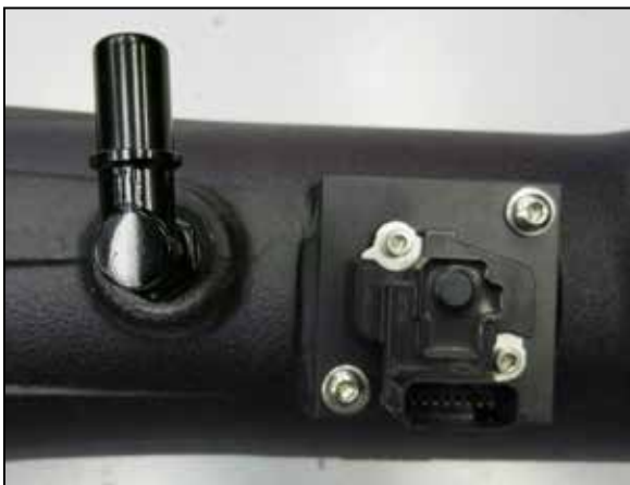
12. Remove the mass air sensor from the factory housing and install it into the K&N adapter using the provided hardware.
