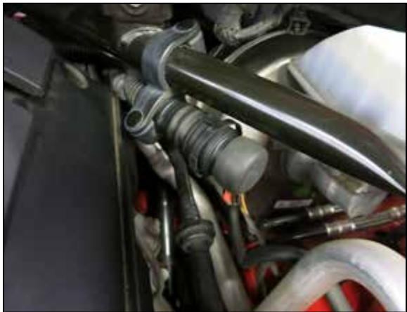
10. Install the quick connect/cap assembly into the remaining sound tube.
