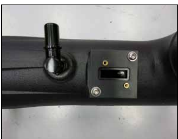
11. Install the provided 90 degree quick connect fitting into the K&N intake tube. Install the provided mass air sensor adapter onto the K&N intake tube using the provided hardware and gasket. Note: The quick connect fitting utilizes 3/8npt threads, thread the fitting in by hand and then tighten one revolution. Be sure to install the mass air sensor adapter in the correct orientation as shown.
