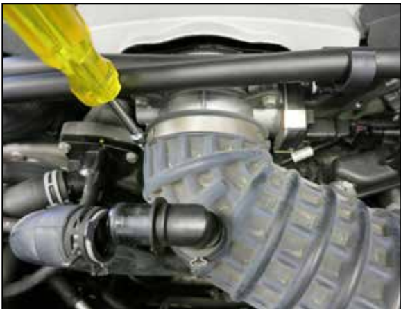
4. Loosen the hose clamp that secures the factory intake tube to the throttle body.
