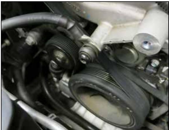
8. Resecure the engine ground with the factory sound drum mounting bolt and crush washer.
