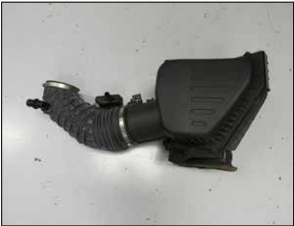
6. Remove the complete factory intake system from the vehicle.
