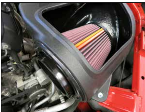
17. Install the K&N air filter into the K&N air filter housing.
