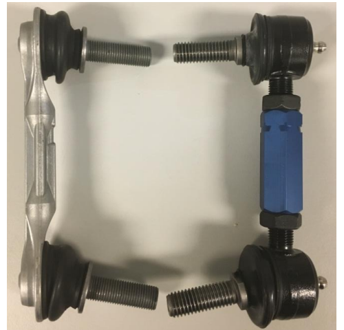
Figure 3: Steeda adjustable rear swaybar endlinks
