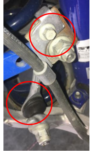
Figure 2: Factory vs Steeda rear swaybar endlinks
