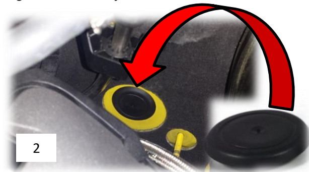
Figure 2: Sound tube plug installed
