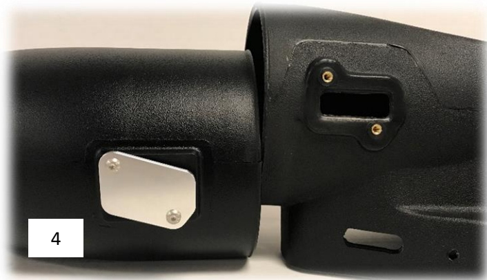
Figure 4: Steeda MAF sensor and block-off plate locations
