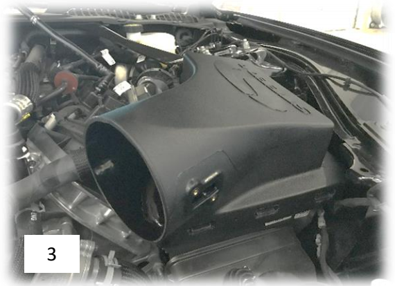
Figure 3: Steeda intake lid installed
