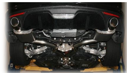
Figure 4 Install clamps on intermediate pipe, do not tighten
