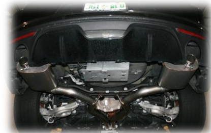
Figure 4 Install clamps on intermediate pipe, do not tighten
