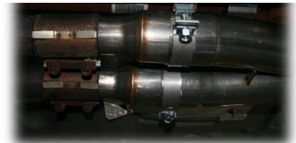
Figure 3 Install provided clamps, do not tighten
