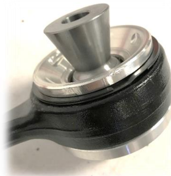
Figure 3: Steeda Front Control Arm Bearing Assembly installed with external snap ring
