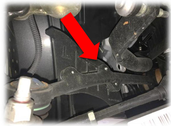
Figure 2: Factory tension link
