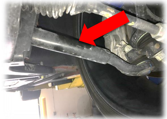
Figure 1: Factory lateral link
