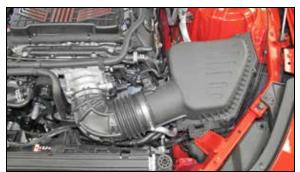
Loosen the hose clamp at the throttle body and then remove the complete stock intake system.
