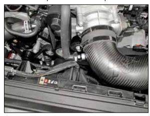
16. Connect the factory crank case vent connector into the quick disconnect fitting installed into the K&N® intake tube.
