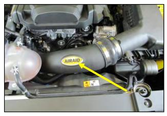
**10.** Insert the large end of the Intake Tube into the Hu Apply the Airaid Bubble Decal onto the Intake Tube as shown.
