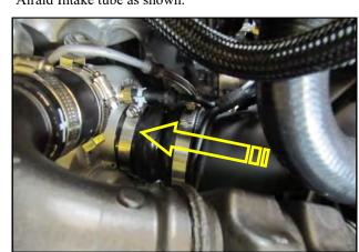
**9.** Lower the Airaid Intake tube down into position and slide the reducer onto the turbo inlet.
