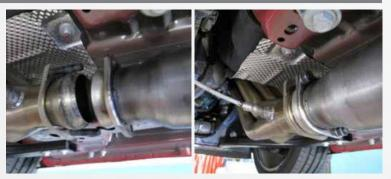
With the BBK Full Length Headers installed on the vehicle lift the BBK Head Pipe into place and bolt it to the collector on the BBK Full Length Header.
