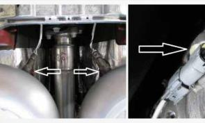
Using a small amount of anti-size on the threads, Install the (2) Oxygen sensors into the BBK Head Pipe Adapters. Run the wiring over the transmission cross member and plug it back into the wiring harness connectors.
