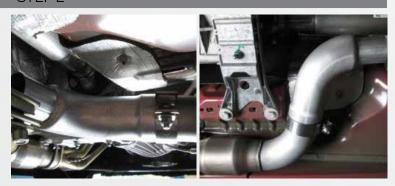
Using the 3" band clamp supplied in the kit slide it onto the BBK Head Pipe Adapter on the flared end then slide it onto the BBK Head Pipe. Rotate the BBK Head Pipe Adapter upward to connect it to the stock location on the resonator.
