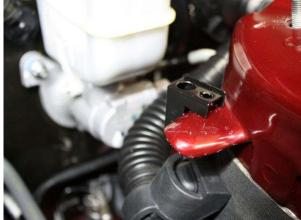
Use the supplied  $\frac{1}{4}$ -20x $\frac{1}{2}$ " bolt and attach JLT Bracket to the black mounting clamp using the smaller hole as shown below:
