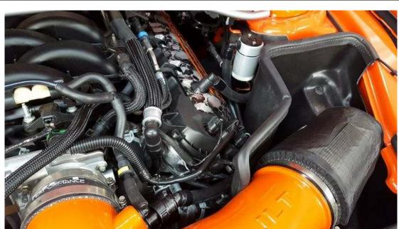
Mount Oil Separator to JLT Bracket with the two supplied machine screws. The longer hose will be closest to the valve cover. Route short hose to valve cover and route long hose to the intake tube.
