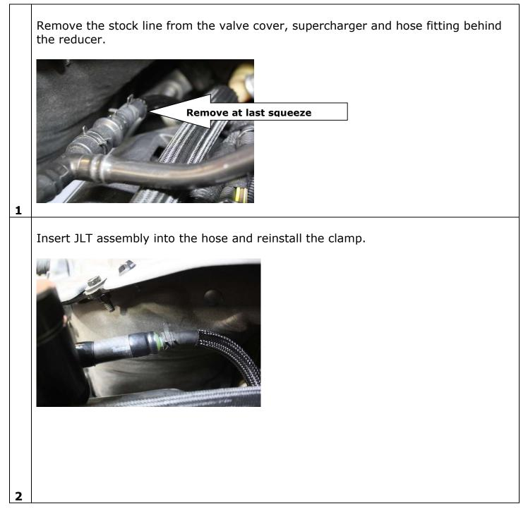
Connect fittings to the valve cover and supercharger and you're done.
