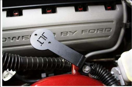
Mount JLT bracket to shock tower tab with supplied nut and bolt
