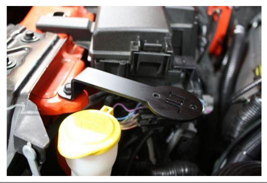
Use the M4x10 screws to attach JLT Separator to the JLT Bracket. Route long hose down and up along the wire harness. Plug on to the fitting on the supercharger and plug the short hose on to the fitting on the valve cover.
