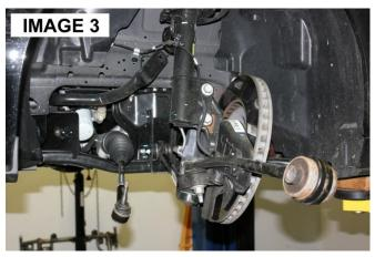
7. Using a ratchet with an 18mm socket and long extension, remove the sway bar saddle bolts on the cradle through the top of the engine bay.
