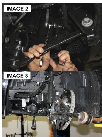
7. Using a ratchet with an 18mm socket and long extension, remove the sway bar saddle bolts on the cradle through the top of the engine bay.
