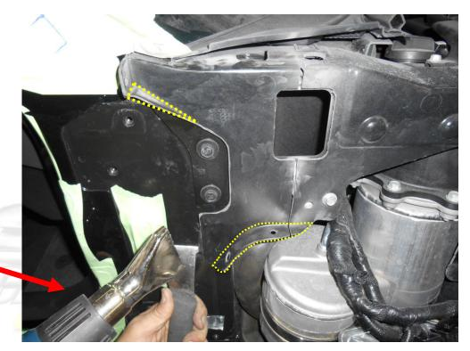
On the passenger's side you will want to remove the ECU to give you more room to work before you trim the fender bracket and install the new VDI Lambo Door hinge.
