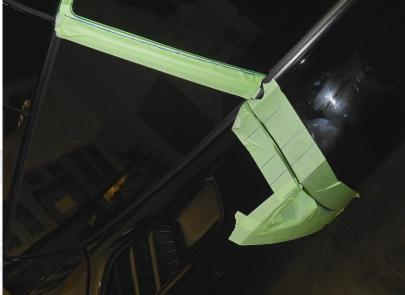
Make sure to measure and mark the distance between the body and the outer door skin at the front of the door by the bottom and top hinge as shown to the right.
