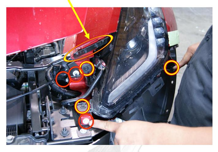
Remove all the bolts securing the headlight to the body. Marked by O circle. After removing the bolts pull forward on the
