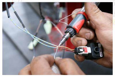
In the image we have removed the sensor to show how to extend the wires but you do not have to remove the sensor, just unplug it.
