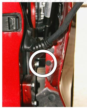
Re-use the OEM speed clip and bolt from the fender bracket that you trimmed off to secure the fender to the supplied fender bracket
