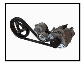
13. Install the new supplied SC belt with the updated routing. Due to eliminating the adjustable idler, belt length is critical. Use the belt guide to help select the belt that works best for your application.
