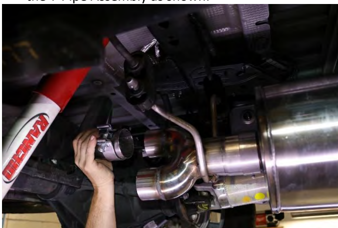
13. Slide the driver's side front tail pipe into the top section of the Y-Pipe as shown.
