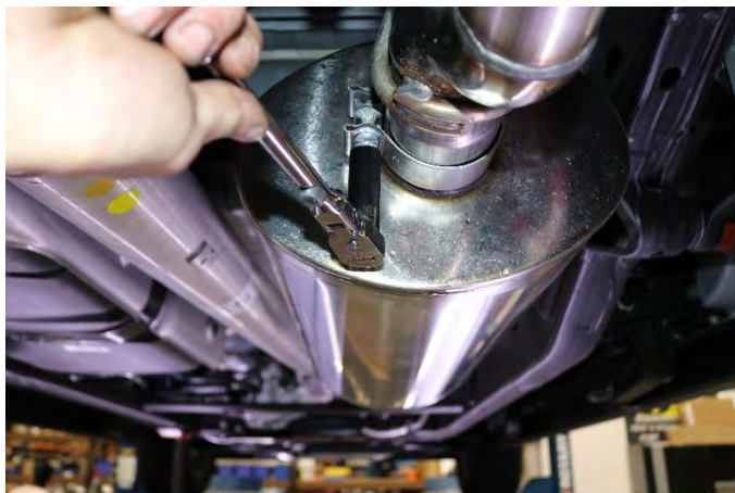
11. Snug the TORCA 3" clamp using a 15mm socket on the Y-Pipe Assembly as shown.
