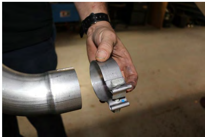
12. Insert a TORCA 2.5" Clamp into the expanded and notched end of the Drivers side Front Tail Pipe.
