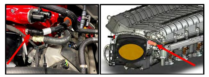
89. Install stock brake aspirator hose from the brake booster to the **lower** quick connect fitting on the supercharger inlet. Push until it clicks into place. **TIP:** For best routing, nestle in between cam cover and fuel rail, under the wiring and heater hose.
