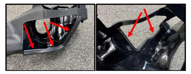
107. Install the supplied rubber strip to ID of air inlet passage on airbox. Butt the two ends at the bottom so its not visible with air-tube installed.
