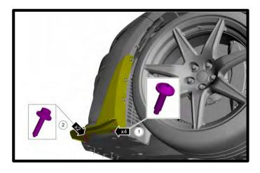
10. Remove the (4) screw covers and (34) retainers from underbody shield.
