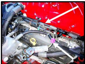
87. Install the (3) supplied 6AN viton oring (#906) to the (3) 6AN to 3/8" quick connect fittings. Install the (1) -6 ORB to 9.89mm fitting to LH top port. Install the (2) -6 ORB to 15.82mm fittings to the LH bottom port and RH port. Use a 11/16" socket to secure.
