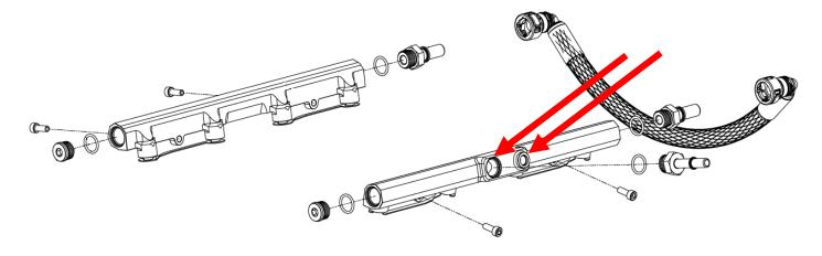
63. Install the supplied (2) #2-908 Viton oring to the (2) -8 ORB to 12.61mm fittings. Apply light amount of grease to oring for ease of installation. Install fittings into rear fuel rail ports. Install the supplied -8 ORB plug to the front fuel rail ports.
