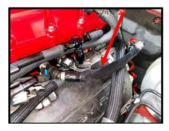
85. Connect the factory fuel PSI sensor connector to sensor, press safety lock until it clicks and locks in place.
