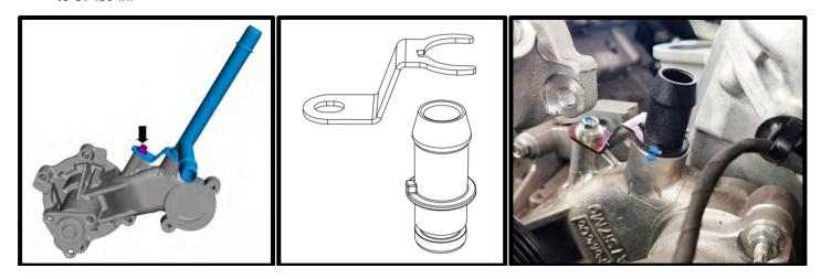
51. Remove water neck from engine by removing the (4) fasteners, this will not be reused. Remove oring from water neck, transfer to new supplied water neck.
