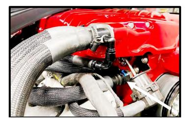
92. (OEM Catch Can) Reuse factory PCV hose and connect to SC inlet 15.82mm quick connect fitting.
