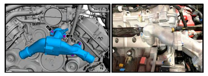
53. Apply light amount of thread sealant to threads of supplied 1/8" NPT to 5/16" fitting. Install fitting into new water neck, rotate to face LH side of engine.
