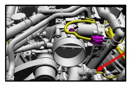
21. Disconnect the EVAP solenoid quick release coupling, release the valve from its bracket, then move out of the way.
