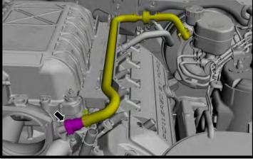
25. Detach the coolant hose and wiring harness retainers, then move the hoses and wires out of the way.
