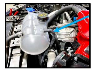
100. Using the previously removed stock TMAP sensor, install stock SIP sensor to Whipple inlet. Apply grease to oring to ease installation. Secure using supplied 5mm x 18mm HHFCS bolt. Torque to 72 in-lbs.
