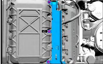
27. Remove the fuel rail insulator from both banks.
