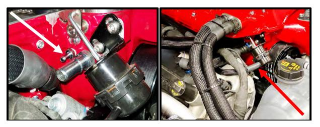
91. **(Non-OEM Catch Can)** Using razor, carefully remove the 90deg and straight fittings from PCV hose. Install the supplied ½" x 7" hose to the stock 90deg and straight ½" quick connect fittings. Install 90deg end to valve cover, straight to supercharger inlet 15.82mm fitting. Push until it clicks and locks into place.
