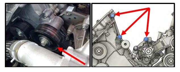
48. Install idler plate to engine with the using the (1) 8mm x 65mm HHFCS, (1) 8mm x 60mm SHCS and (1) 8mm x 55mm SHCS bolts to secure to timing chain cover. Leave loose for now.
