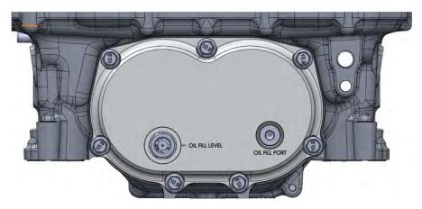
71. Install the supercharger housing (without lid) to the engine. Use the supplied (4) 6mm x 55mm HHFCS on the outer bolt holes and the (6) 6mm x 80mm HHFCS bolts with the supplied (6) #2-009 orings on the bolt, under the head. Use **Blue Loctite #243** on the threads of each bolt. Leave hand tight for now.
