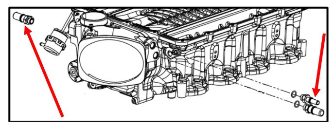
88. Install the supplied 3/8" ID x 5 ½" with 55deg quick connect fitting hose (#5000030) to the EECPV barb fitting and **upper** quick connect fitting on SC inlet. Push until it clicks and locks into place.
