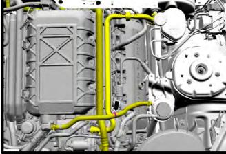
26. Remove the (6) nuts from SC lid, then remove the hose supports from both sides.
