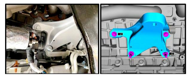
42. Install the new passenger side motor mount bracket using supplied (2) 10mm x 30mm HHFCS bolts to the top bolt holes. Secure bottom using the stock studs, the (2) .835" spacers (1 per stud), the stock bracket and ground eyelet as stock. Torque to 41 lb-ft.
