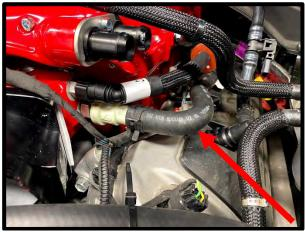
90. Apply light amount of pipe Teflon to supplied 1/8" NPT to ¼" barb fitting. Install fitting to the open port on the SC inlet (vacuum source). Install the supplied ¼" ID premade hose to the bypass actuator barb and ¼" fitting on SC inlet. **CAUTION:** Verify hose can't kink or bend.
