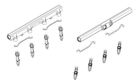
65. Apply generous amount of grease to the injector orings for ease of installation. Install the fuel injectors, rails and lock bracket to the intake manifold, secure with the (4) 6mm x 16mm SHCS using a 5mm allen socket. Use **Blue Loctite #243** on the threads of each bolt. Torque to 90 lbs-in.
