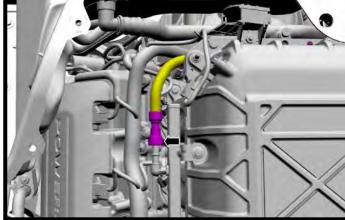
30. Detach the retainer securing fuel line to SC assembly, then remove fuel line from engine.
