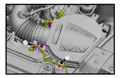
19. Disconnect the crank case vent tube and bypass vacuum line from inlet tube. Loosen clamp at throttle body. Remove the airbox mounting bolt and remove airbox assembly.
