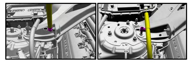
16. Remove the (2) bolts from the supercharger degas bottle bracket and push aside (8mm socket).
