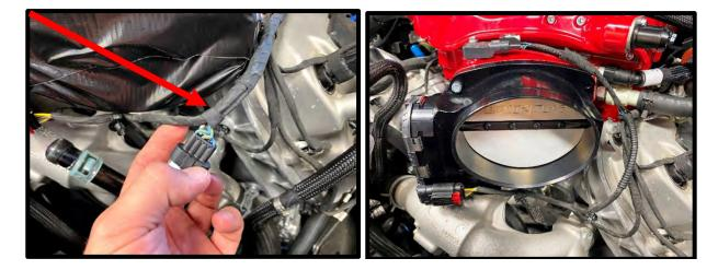
103. Install supplied 1.0625" OD (3/4" ID) rubber grommet into air inlet tube. Install stock air temp sensor into supplied plastic adapter. Insert air inlet temp sensor into air tube
