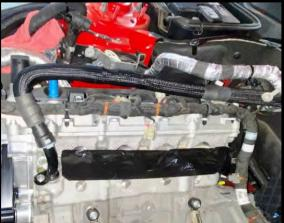
57. Install the supplied tee and 90deg hose to the driver side heater tube you just installed. Secure with the supplied (2) #10 clamps.
