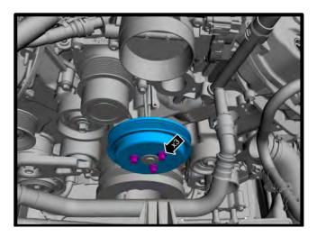
38. Remove the supercharger from engine by removing the (6) supercharger assembly bolts and (4) bolts from fuel rails (10mm socket).
