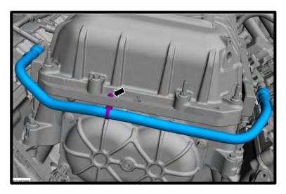
31. Detach wiring harness retainers (3) from SC assembly and push aside.
