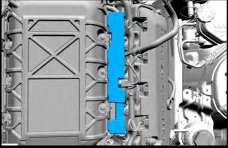
28. Disconnect the quick release coupling from degas bottle. Remove hose from engine, this will not be reused. Disconnect coolant quick release from upper heater tube. Remove vent line from degas bottle and water neck, this will not be reused.
