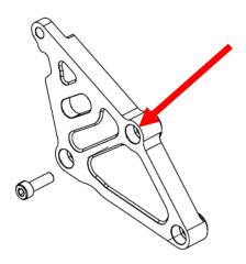
73. Torque the (10) 6mm HHFCS manifold bolts in the following pattern using a 10mm socket. First pass: 88 lbs-in. Second pass: 106 lb-in. **NOTE:** For bolt #10, a ¼" socket with 4"-6" extension, 10mm wobble is the best possible tool to get into this tight area.
