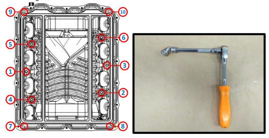
74. Torque the (3) idler plate bolts that secure plate to timing cover and plate to inlet, to 21 ft-lb. Torque the (1) 8mm x 55mm SHCS bolt to water pump to 180 in-lb.
