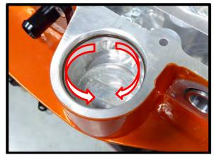
83. Apply generous amount of grease to the (1) #2-230 Viton bypass oring. Install the supercharger lid to the supercharger housing by carefully placing the bypass down. Secure the SC lid using the (17) 6mm x 30mm HHFCS and (3) 6mm x 70mm HHFCS (*marked green*) using the following pattern. Torque to 90 lbs-in using an 10mm socket.
