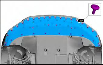
11. Remove the (10) retainers and (4) push pins from underbody shield. Remove underbody shield from vehicle.
