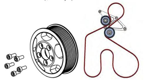
79. With the belt holding the SC pulley in position, torque the supercharger (5) 6mm x 14mm SHCS bolts to 130 lbs-in using a 5mm allen socket. Do not use Loctite on threads, it is not required.
