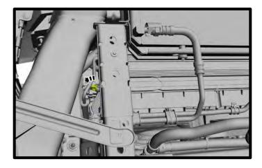
13. With a cool engine, drain the intercooler coolant into a clean drain pain for later reuse.
