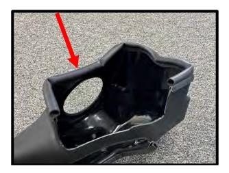
106. Install the 90deg weather stripping to bottom edge of airbox opening (seals to inner fender).
