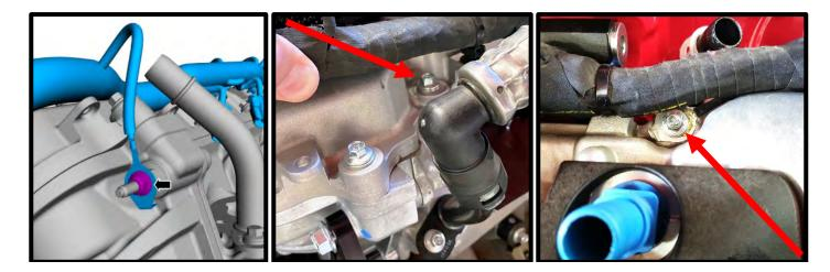
35. Loosen the coolant pump pulley bolts (10mm socket).
