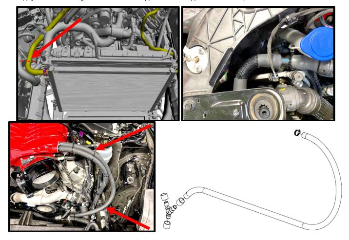
97. Install supplied 23" hose sheaving and (2) heat shrink tubing over stock IC inlet hose, once shrunk, install to RH rear IC fitting (inlet). Secure with supplied black worm clamp (16-27mm).
