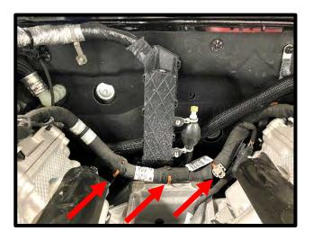
46. Remove the plastic harness retaining assembly from wiring. Remove the trans bladder retainers (2). Using a cut off wheel or saw, remove the tab from bracket to clear new supercharger. Reinstall transmission bladder and plastic assembly to wiring harness. Secure by reclipping and using black automotive grade electric tape.
