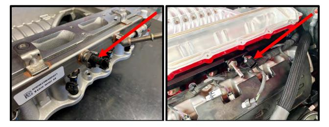
62. Install the supplied (1) #2-906 Viton oring to the (1 of 2) 45mm long -8 ORB to 9.49mm inlet fitting next to fuel PSI sensor. Apply light amount of grease to oring for ease of installation.
