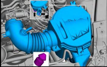
20. Disconnect throttle body electrical connector and coolant temp sensor, then detach the wire retainer.
