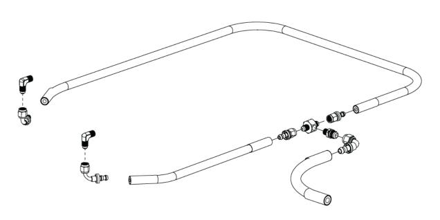
95. Install the supplied ¾" x 18 ½" hose to the LH front IC fitting (outlet), secure to IC fitting using supplied black worm clamp (16-27mm). Pre-install (2) 1" x 2" heat shrink tubing and the 23" sleeve. Locate the outlet hose from degas bottle and cut hose as shown. Install the Y fitting to the IC hose and degas outlet hose. Use Gates shrink clamps to all three ends of Y. Use heat gun to shrink clamps, sleeve and heat shrink.
