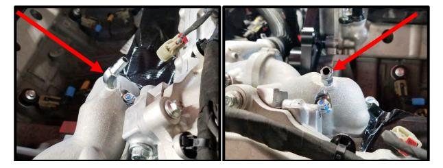
54. Preinstall supplied vent hose (#3103098) to the 45deg fitting in water neck, secure using stock clamp. NOTE: This will later be routed to engine degas bottle.
