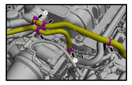
24. Disconnect the PCV line from RH valve cover and SC. Disconnect brake vacuum hose connector from SC and position aside the hose.
