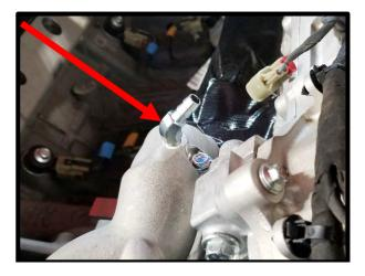
55. Remove stock coolant temp sensor from factory thermostat housing. Install supplied plug to factory location. Install coolant temp sensor in new water neck (needed for throttle body clearance).
