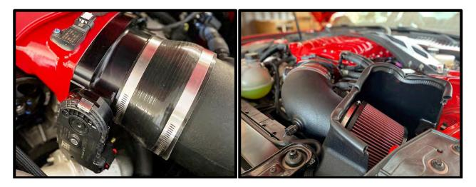
109. Install the ½" ID rubber grommet to air tube port. Connect supplied ½" x 2 5/8" rubber hose. Connect to stock crank case pressure sensor. Connect other end to ½" barb at inlet tube.
