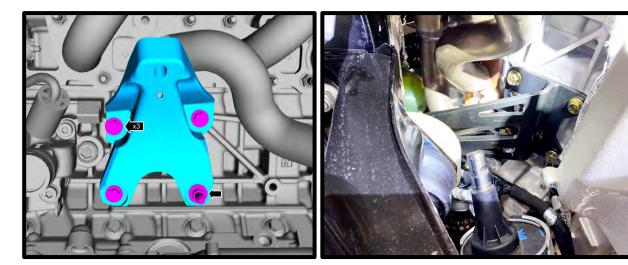
44. The bracket lowering equals ½" lower than stock. Lower engine until it sits on the new motor mounts. Install supplied thick washer to factory mount studs (1 per). Install stock upper mount nuts. Torque to 46 lb-ft.
