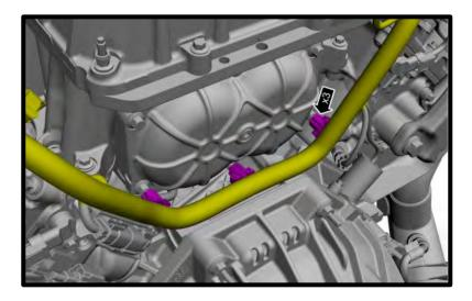
32. Disconnect the TMAP sensor from supercharger lid and TMAP (SIP) sensor from supercharger inlet. Remove both sensors from supercharger assembly for installation to new supercharger. **NOTE:** Do not mix up sensors.
