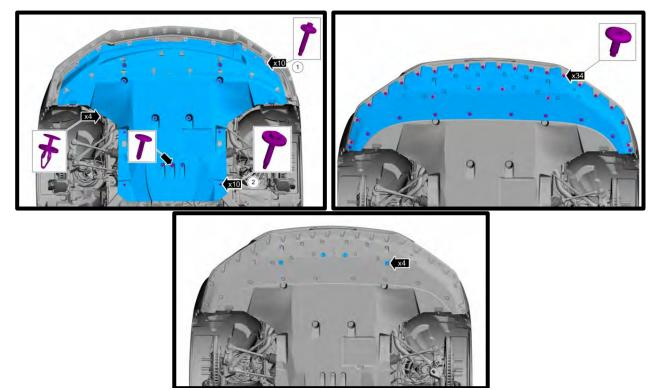
111. If equipped, on both sides, position the splitter wicker and install using stock retainers. Torque to 53 in-lbs.
