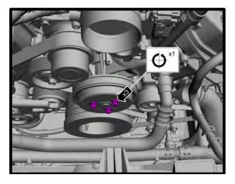
36. Rotate the accessory drive belt tensioner counter clockwise and remove belt. Rotate the supercharger belt tensioner clockwise and remove supercharger belt. Remove belt from engine.
