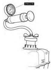
118. To pressurize the cooling system, slowly press the plunger of the pressure test pump and increase the pressure to between 124 - 138 kPa (18 - 20 PSI). Observe the gauge reading for approximately 2 minutes. Pressure should not drop during this time. If the pressure drops within this time, inspect for leaks and repair as necessary. **NOTE:** If no leaks are found and the pressure drops, the leak may be internal to the intake manifold.
