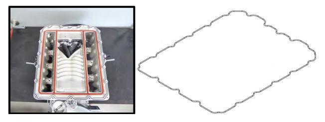
82. Install the (1) #2-230 internal bypass oring to the lid bypass passage. Use generous amount of grease to secure oring in place.
