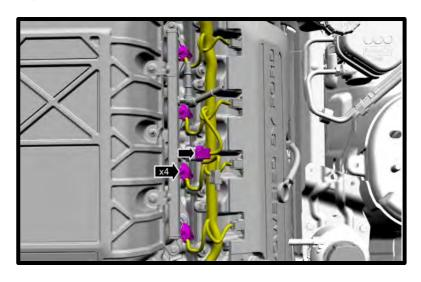
34. Remove factory ground wire by removing nut, using 10mm wrench. Relocate to valve cover bolt. Torque to 89 in-
