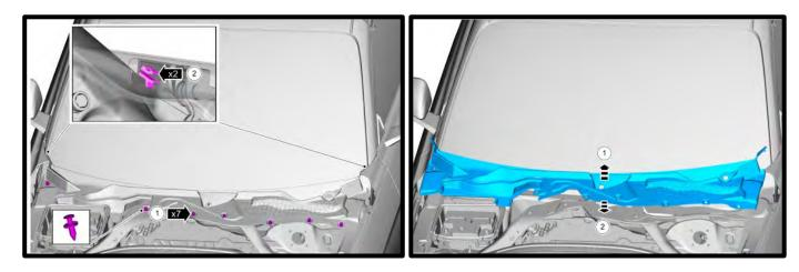
15. Safely support the hood with a hood prop. Disconnect the lower hood support. Detach wiring harness retainer from strut brace.
