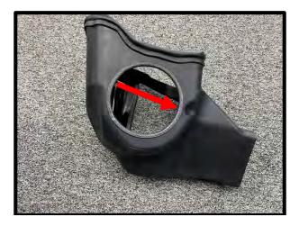
108. Install the airbox to the stock location. Install air tube and air filter to end of tube. Secure filter using supplied clamp. Connect air tube to throttle body using the 5.50" x 5.00"" coupler. Secure using #80 (TB) and #88 (air tube) hose clamps. Connect 2-way IAT connector to sensor.
