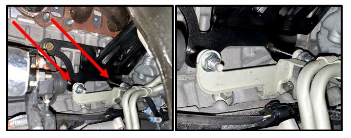
43. Using a 13mm socket, remove the (3) bolts and (1) stud bolt from driver side engine bracket. Install supplied bracket to engine, secure with the (4) 10mm x 30mm HHFCS bolts. Torque to 41 lb-ft.
