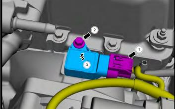
33. Disconnect all (8) fuel injectors and fuel pressure sensor electrical connectors.
