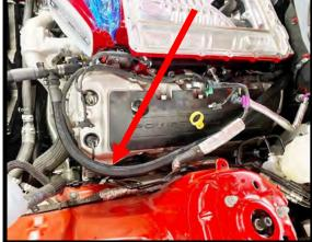
59. Install the supplied 3/4" x 15" coolant degas hose to the new supplied tee fitting. Slide the 18" hose sleeve over the hose, along with (2) 1" x 2" heat shrink tubing. Secure new hose using stock pinch clamps. Use a heat gun to lightly shrink sleeve to hose and shrink heat shrink tubing to end of sleeve. Use adel clamp to front bolt of thermostat housing to secure hose. Torque to 89 in-lbs.
