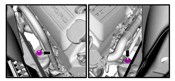
41. Remove the (2) upper bolts and (2) nuts from bottom of engine mounts (studs will be reused on lower holes).
