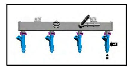
61. Using a 24mm socket, remove the fuel PSI sensor from the factory fuel rail. Using a 24mm socket, remove the fuel PSI sensor from the factory fuel rail. Install the factory fuel PSI sensor to the fuel rail using a 24mm socket. Torque to 53 lbs-in, then an additional 25-degree rotation. **NOTE: No sealant on the threads.**
