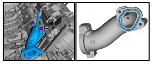
52. Install new water neck into stock location. Secure to cylinder head using the (1) 6mm x 30mm and (1) 6mm x 50mm SHCS. Secure to stock thermostat housing using factory fasteners. Get all parts hand tight before torquing. Torque the (2) nuts to 89 in-lbs first. Follow by torquing stock water neck bolts to 89 in-lbs.
