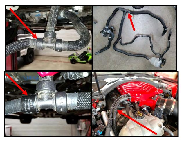
99. Install the new supplied vent hose (#3103098), from the 45deg fitting in water neck, to engine degas bottle. Secure both ends using stock hose clamps. Secure hose with zip ties to previously routed degas bottom 3/4" hose.
