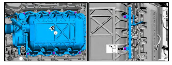
39. Remove the (2) nuts securing plastic harness assembly to SC and engine, position aside for later modification (10mm ratchet wrench).
