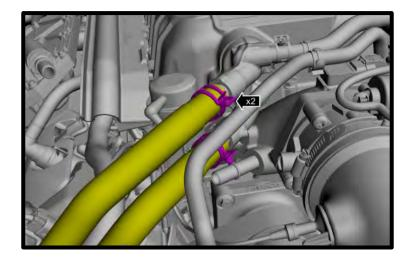
23. (1) Disconnect the hose clamp and the retainer, then position aside the hose. (2) Disconnect the supercharger cooling circuit hose clamps and retainers. These hoses will not be reused.
