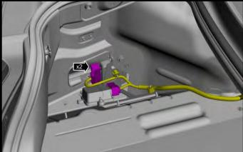
6. Remove the (3) retainers from battery cover and remove cover. With an 8mm wrench disconnect the (-) negative battery cable. Make sure the cable is far enough away from the battery that it does not accidentally touch the battery and make connection during the installation.
