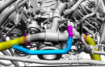
29. Disconnect the fuel supply quick release coupling from fuel rail. Disconnect the fuel rail cross over hose using a 3/8" fuel line removal tool.
