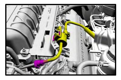
22. Mark each factory intercooler hose for future reference. Top is outlet, bottom is inlet. Remove both hoses from barbs and push aside.
