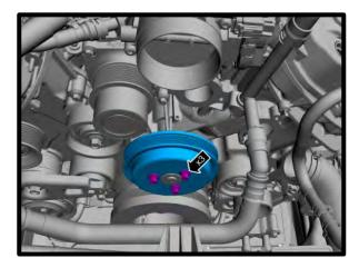
77. Reinstall stock accessory belt by releasing tension on spring loaded tensioner.
