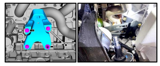
6. The bracket lowering equals ½" lower than stock. Lower engine until it sits on the new motor mounts. Install supplied thick washer to factory mount studs (1 per). Install stock upper mount nuts. Torque to 46 lb-ft.
