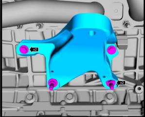
4. Install the new passenger side motor mount bracket using supplied (2) 10mm x 30mm HHFCS bolts to the top bolt holes. Secure bottom using the stock studs, the (2) .835" spacers (1 per stud), the stock bracket and ground eyelet as stock. Torque to 41 lb-ft.
