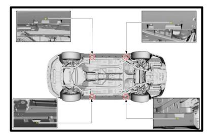
3. Remove the (2) upper bolts and (2) nuts from bottom of engine mounts (studs will be reused on lower holes).
