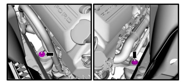
2. Lift the vehicle using the Ford recommended lifting points and place on to safety stands.
