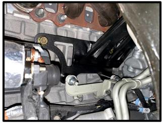
5. Using a 13mm socket, remove the (3) bolts and (1) stud bolt from driver side engine bracket. Install supplied bracket to engine, secure with the (4) 10mm x 30mm HHFCS bolts. Torque to 41 lb-ft.
